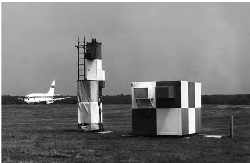
Microwave Landing System hardware at NASA's Wallops Flight Research Facility in Virginia as a NASA 737 prepares to take off to test the high-tech navigation and landing aid. NASA.
