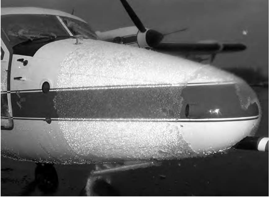
Post-flight image shows ice contamination on the NASA Twin Otter airplane as a result of encountering Supercooled Large Droplet (SLD) conditions near Parkersburg, WV.
