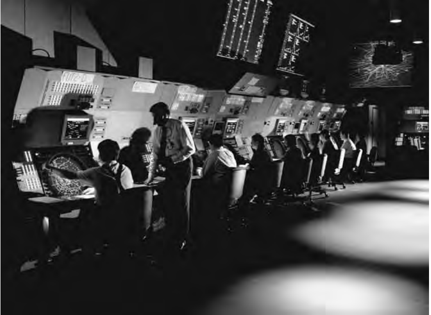
Flight controllers test the Traffic Manager Adviser tool at the Denver TRACON. The tool helps manage the flow of air traffic in the area around an airport. National Air and Space Museum.
