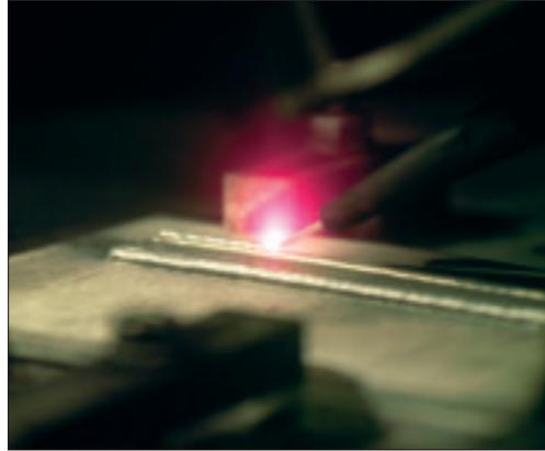
An electron beam free form fabrication is shown at work laying down a metal part one layer at a time. The EBF<sup>3</sup> process allows for more intricate components to be manufactured using smaller amounts of raw materials than conventional methods use. Image credit: NASA.
