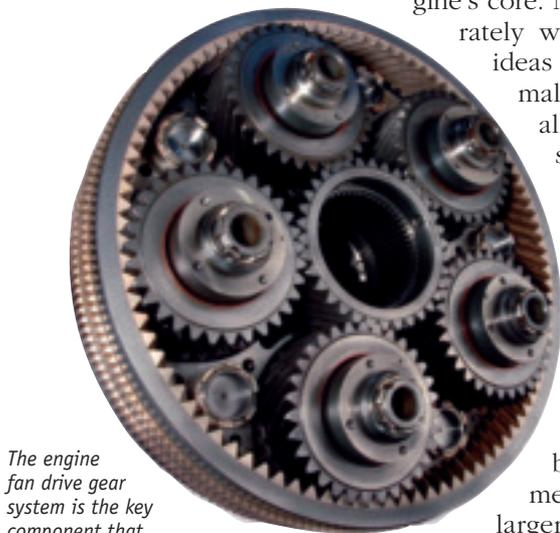
*The engine fan drive gear system is the key component that makes it possible for the P&W geared turbofan engine to work and thus to increase the engine's fuel efficiency. Image credit: Pratt & Whitney.*
