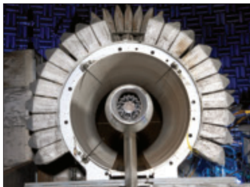
A view upstream looks into the NASA/Rolls-Royce variable-cycle nozzle with a lobed mixer, mounted on the jet rig in the Nozzle Acoustic Test Rig during acoustic testing in the AeroAcoustic Propulsion Lab at NASA Glenn.
