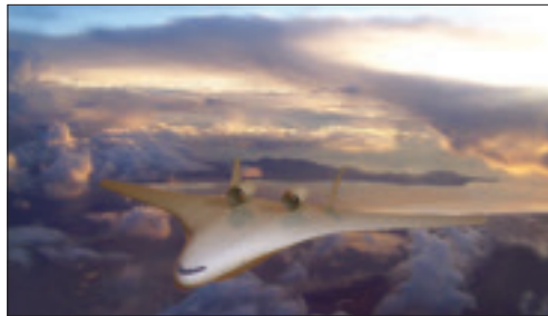
This hybrid wing body concept (N2A HWB) has the engines mounted on top of a body that deflects noise upward instead of toward the ground. The concept was generated by Boeing under a Subsonic Fixed Wing Project study and is planned for testing in 2012 by NASA's Environmentally Responsible Aviation Project. Credit: NASA.
