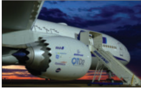
NASA has partnered with industry many times during years of chevron testing, including these tests of nozzles on a specially adapted GE engine mounted on a Boeing 777. Chevron nozzles will be seen on more engines in the coming years. Credit: Boeing/Bob Ferguson.
