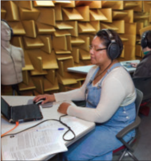
Gold-colored foam wedges shield test subjects from outside noises during an acoustics test at NASA Langley. NASA researchers study people's perception of aircraft sounds in an indoor setting and investigate the role of rattle noises and vibration. They use this information to help design quieter aircraft. Credit: NASA Langley/Sean Smith.
